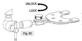
**05- Dentulous bitefork (12):** Position the bitefork in the transfer set until the transfer set limit and use the screw to fix it (fig.05).
